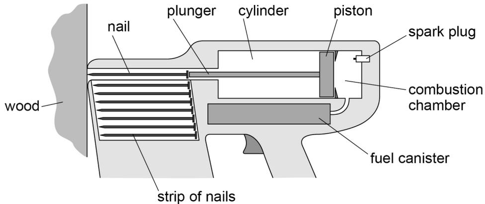
Fuel is mixed with air in the combustion chamber and is ignited by a spark. The gas expands rapidly and drives the piston along the cylinder. The plunger attached to the piston drives the nail into the wood.
