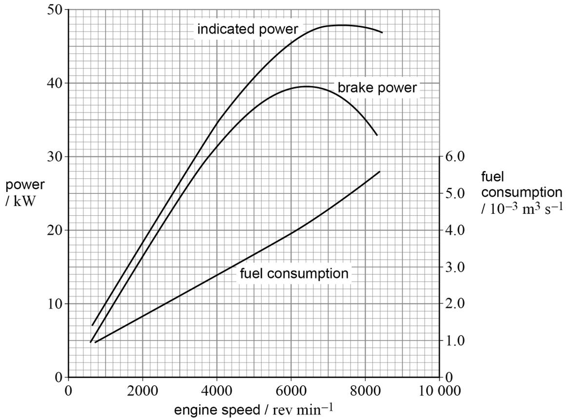
**Figure 4** shows how the indicated power, brake (or output) power and fuel consumption of the engine vary with the engine speed. The scale on the left-hand axis is power and the scale on the right-hand axis is fuel consumption.
