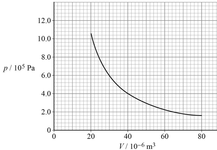
The combustion chamber has a volume of  $20 \times 10^{-6} \text{ m}^3$  and the piston moves through a volume of  $60 \times 10^{-6} \text{ m}^3$ .
